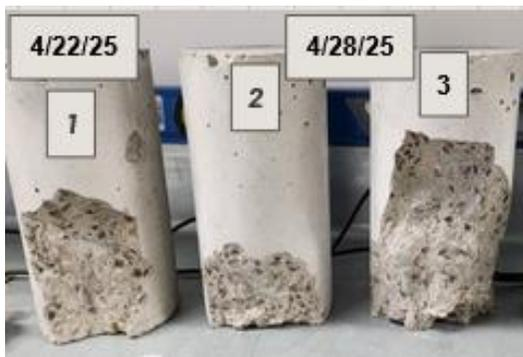
Figure 5: Cylinder Test Breaks with dates and labels corresponding to Table 5
