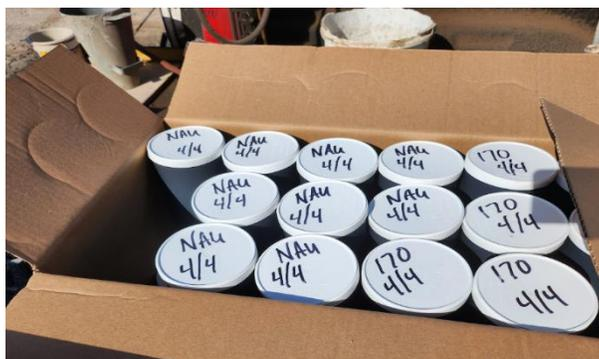
Figure 17: Fabricated test cylinders in molds
