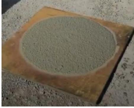
Figure 16: Spread Test results
