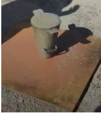
Figure 15 (left): Spread Test set up
